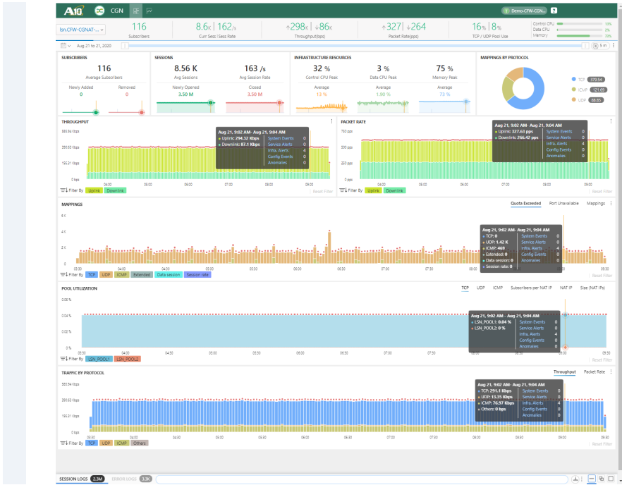
Figure 10. CGNAT App provides comprehensive visibility and insights of the subscriber traffic on a per-CGNAT service basis.
