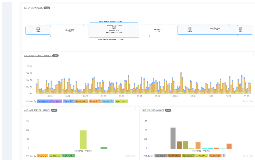
Figure 7. Latency drilldown analytics provides time-series average end-to-end latency for a full request-response cycle. This greatly helps troubleshoot application performance issue related to delayed response time.
